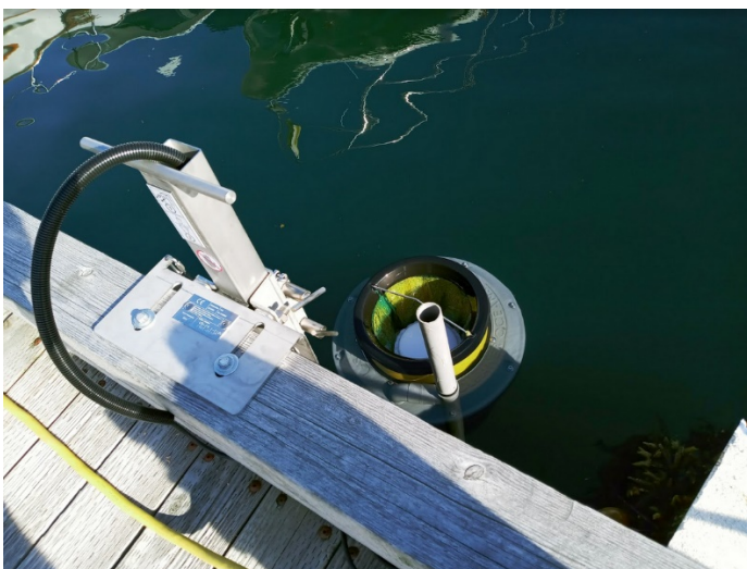
Figure 1. Seabin fully operating at Deer Harbor Marina. Photo Credit: R.P. Oates
