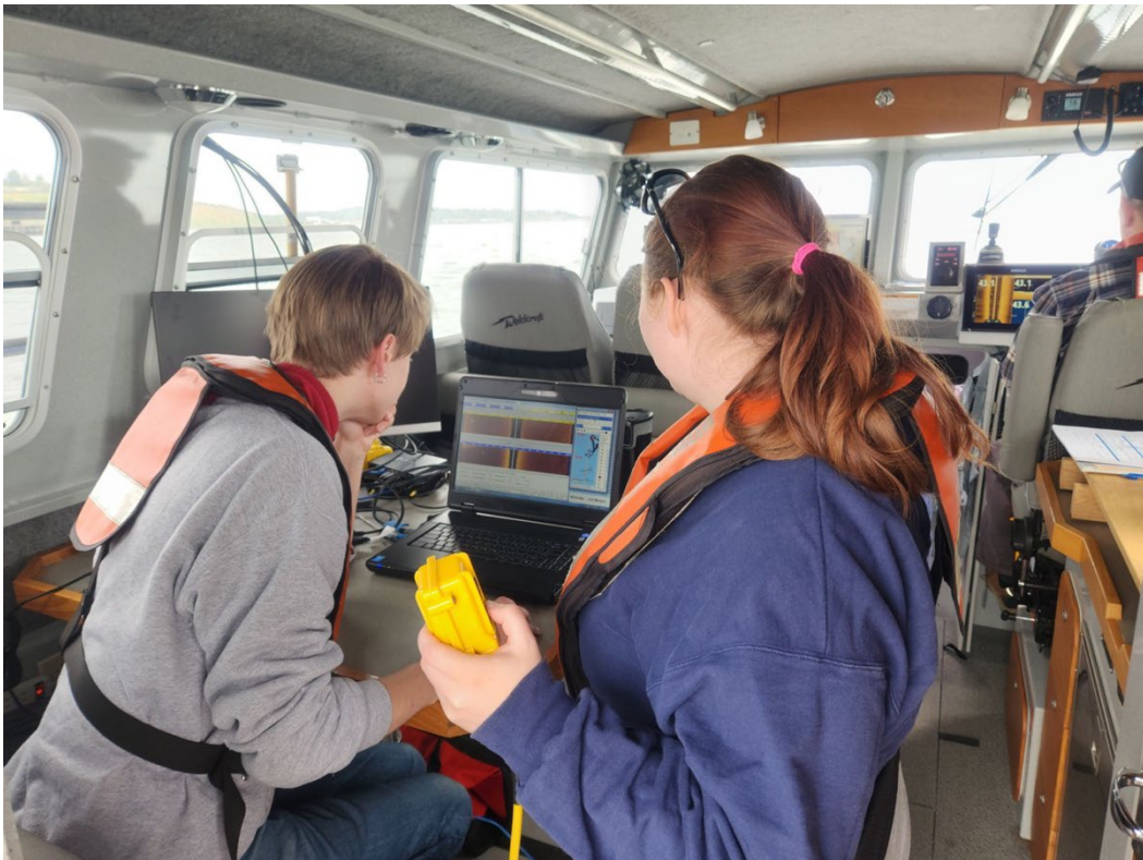
Oscar (Sea Dragon) prepping to mark potential derelict crab pots as Amelia (MRC Assistant intern) controls the winch to adjust the depth of the side scan sonar.
