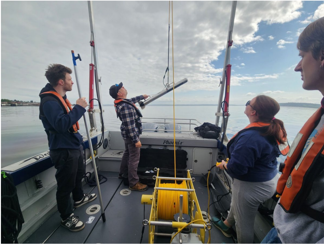
Logan (Sea Dragon), Ben (Coastal Sensing & Survey), Amelia (MRC Assistant intern) and Oscar (Sea Dragon) deploying the side scan sonar.
