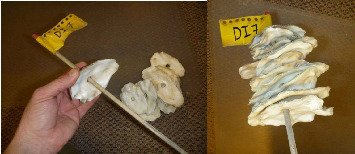
Figure 4. Shell-string collector assembly.
