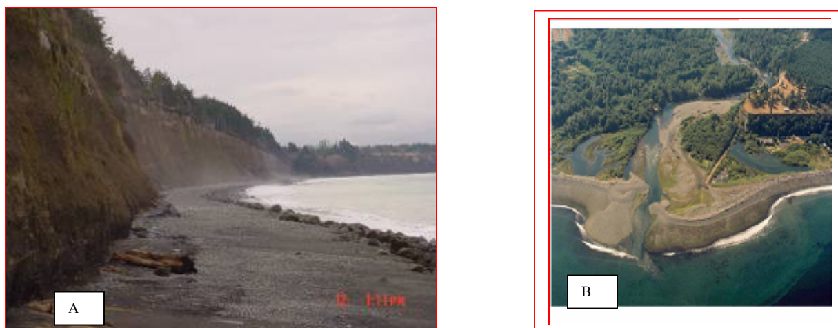
Figure 2. Elwha nearshore limiting features: A. Bulkhead along feeder bluffs; B. Dike on west river mouth.
