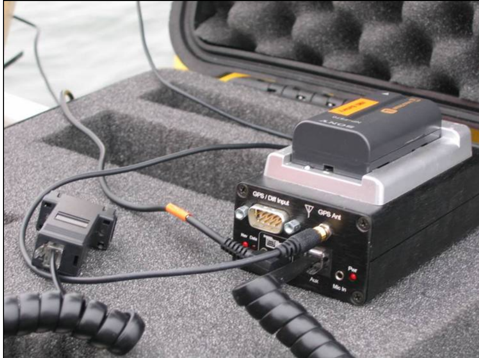
Figure 1. VMS 300 unit consisting of a lithium battery, feature trigger, GPS antenna, and 3.5mm stereo cable for attaching to the video camera.
