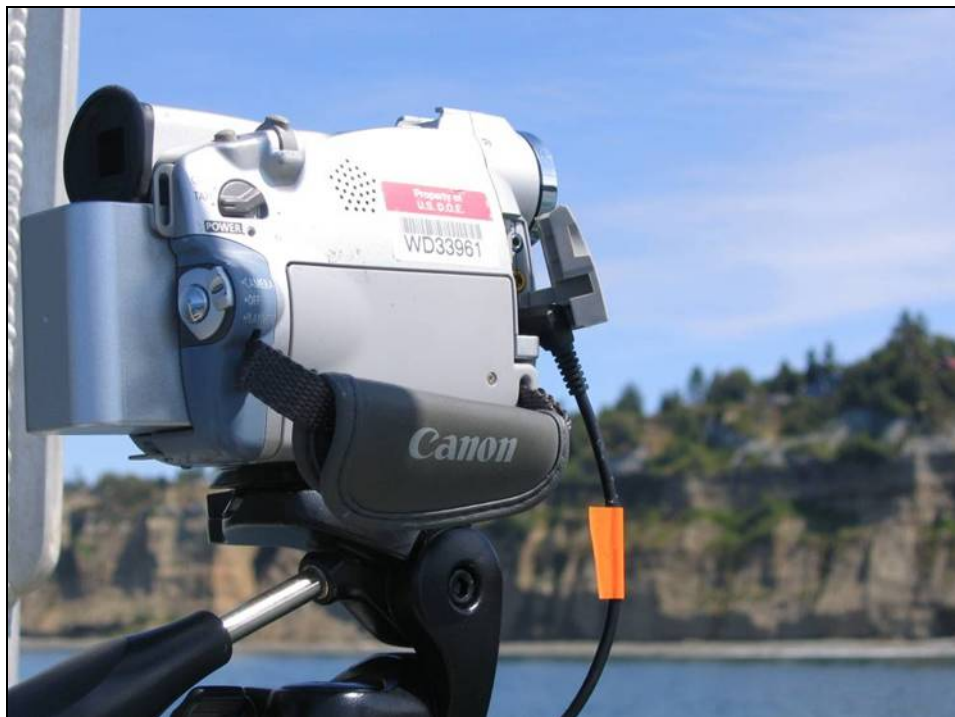
Figure 2. Canon ZR45 MC Digital Video Camcorder with the 3.5mm stereo cable between the VMS 300 microphone/headphone connector and the video camera's microphone input connector.
