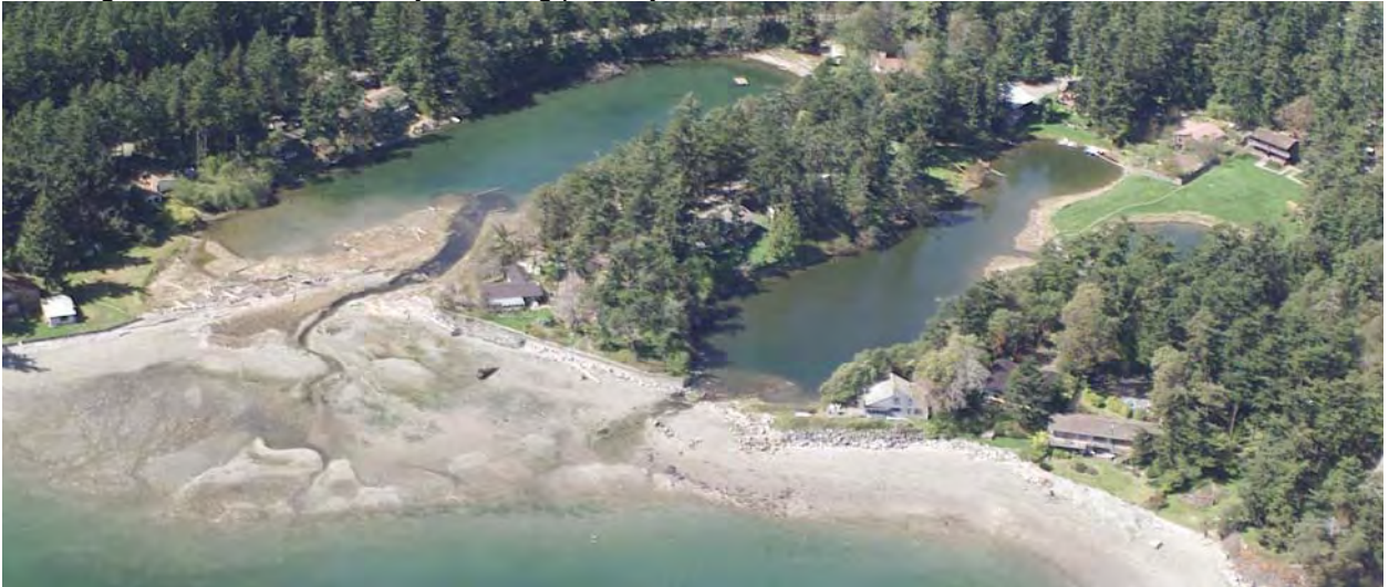
17 Lagoon-restore tidal flow by widening partially filled inlet
