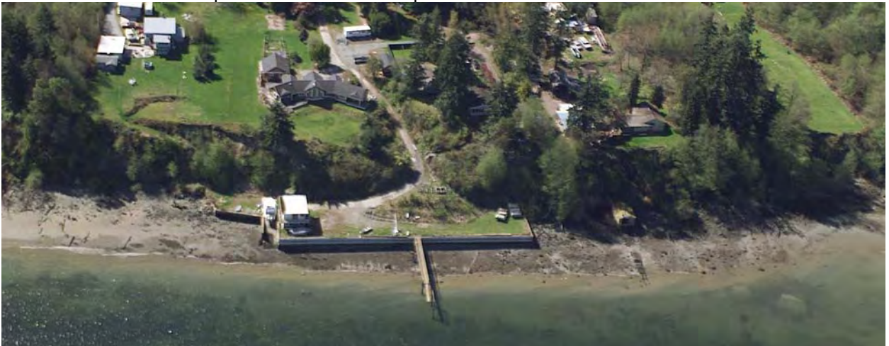
40 Remove PVC sheet pile and creosote wood pile wall and fill and house
