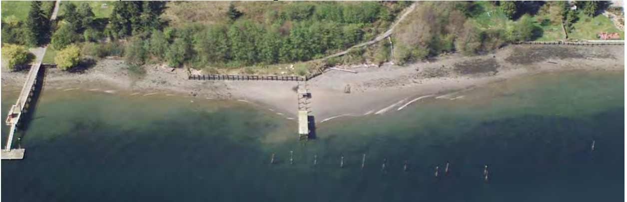
43 Remove failed pier and fill area with failing bulkhead
