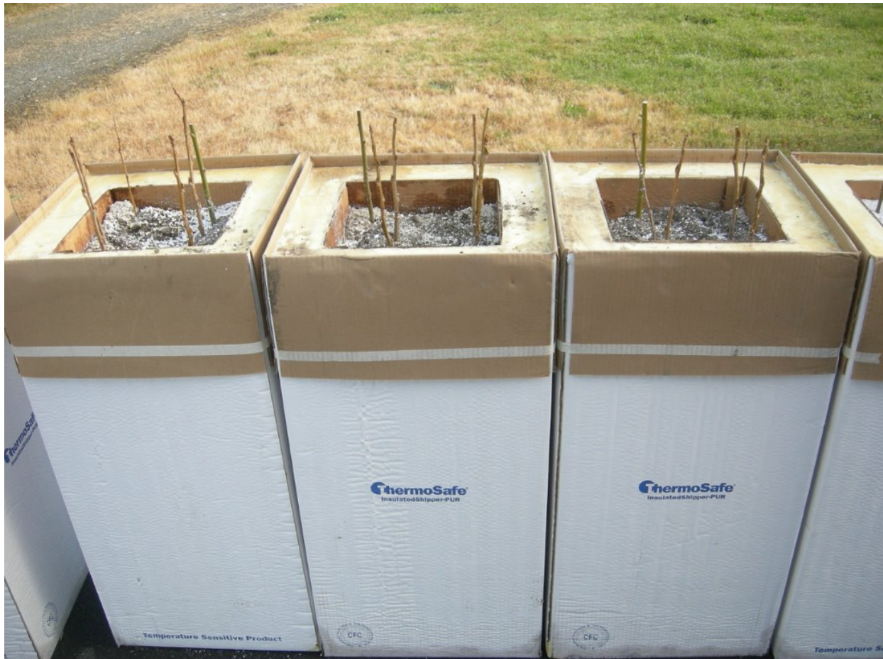
Figure 2-1. Phytobox setup containing perlite-only with trees planted.
