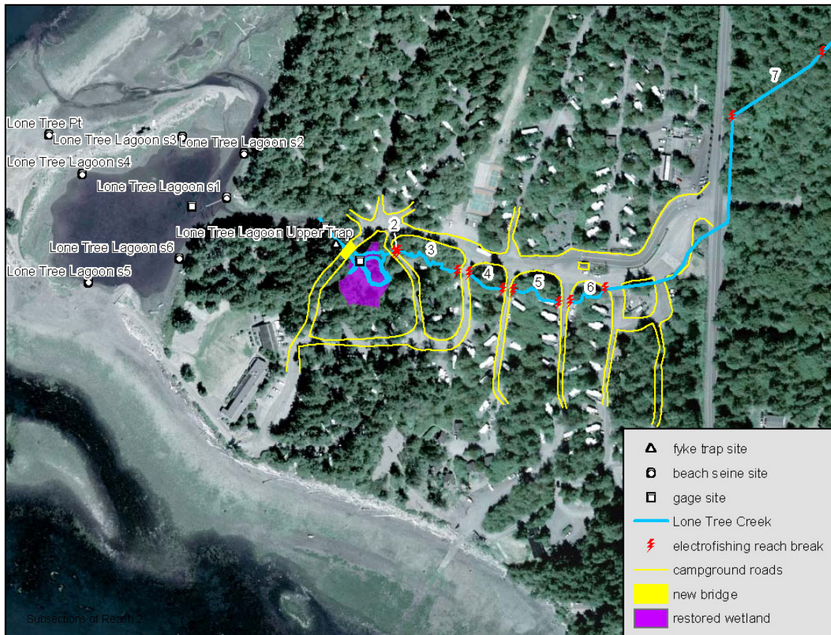
Figure 2. Location of new bridge (and culvert removal site), restored drowned channel wetland, and fish monitoring and tidal water surface elevation gage sites. Numbered spots mark electrofishing reaches.
