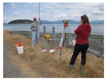
March Point measurements to improve accuracy of baseline survey with level on USACE benchmark shooting to reference point 148 for start point of beach profile.
