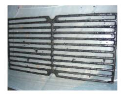
Propane grill grate with months of baked-on food, shown at left. Same grate, right, after soaking in washing soda solution for 24 hours and light scrubbing
