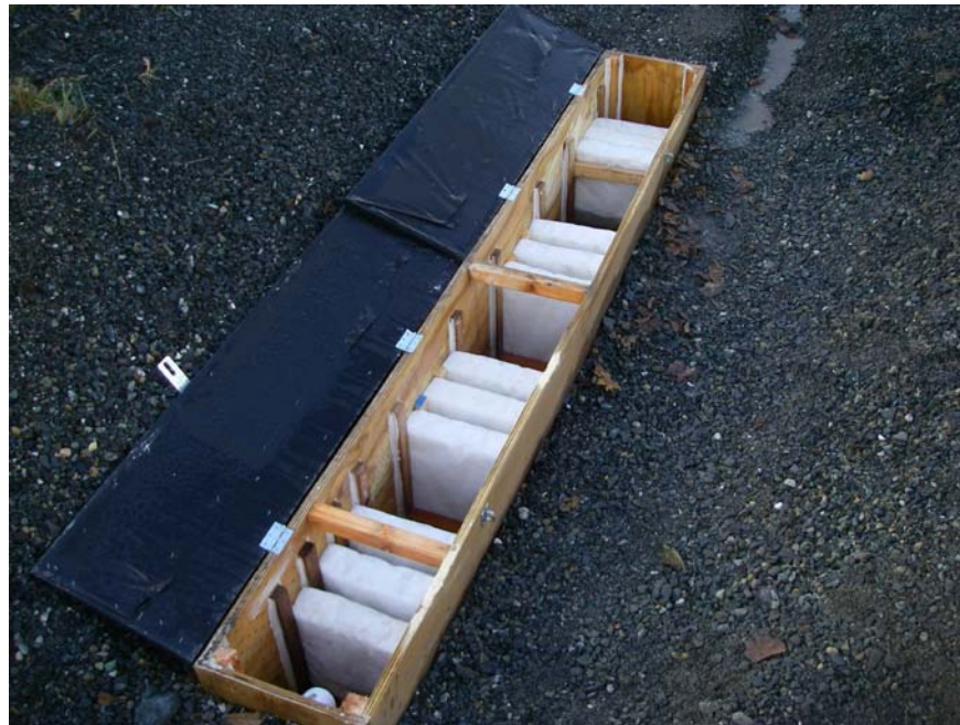
Figure 3. The SWAT experiment trough with the Smart Sponge ® Paks installed. The design allows the water to flow through up to 12 Paks. If the leading Paks clog due to sedimentation, then the storm water will flow over the clogged Paks to the next sets.
