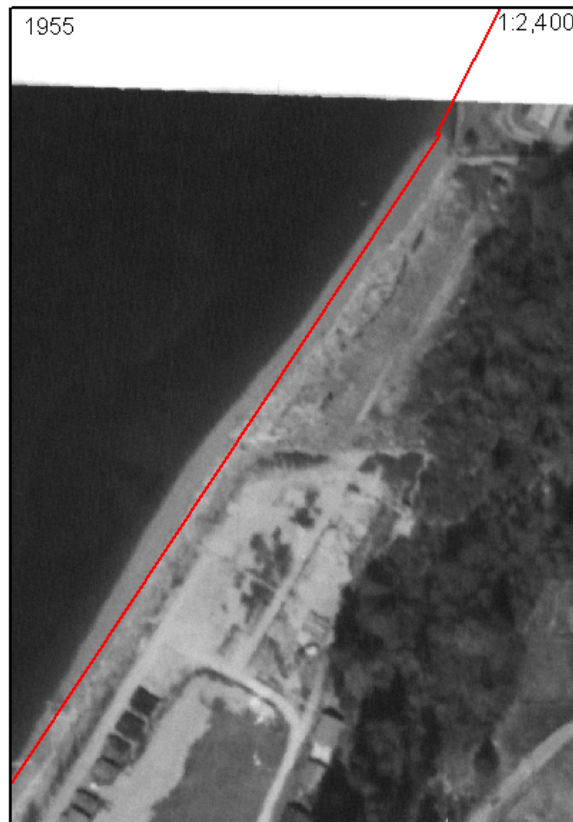
Figure 12. 1955 air photo of the north shore of Kayak Point County Park. Note changed configuration of fill area, narrower driftwood deposit, and installation of shore modification along northernmost shore. Photo courtesy of Snohomish County.
