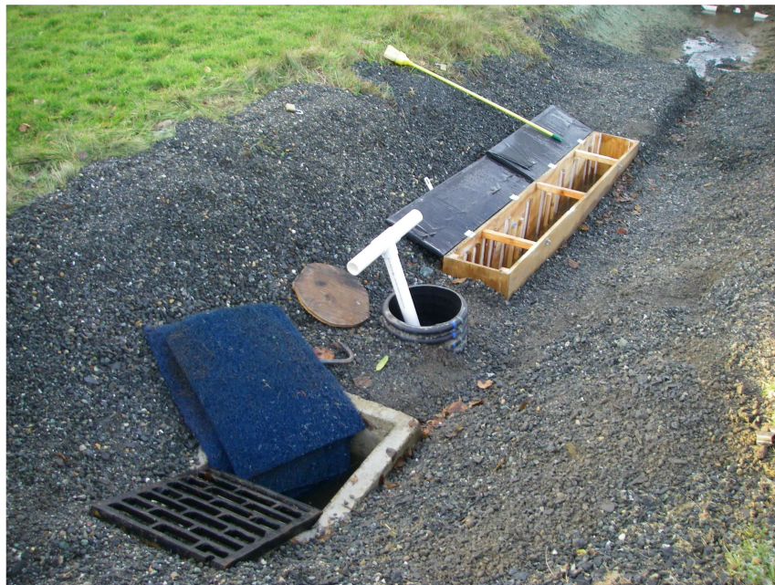
Figure 2. Detail of the SWAT experimental unit installed at Bay View. The sediment retention sump (with filter material) is in the foreground. In the middle is the well holding the 2" PVC flow control valve and the SWAT experimental trough is in the background.
