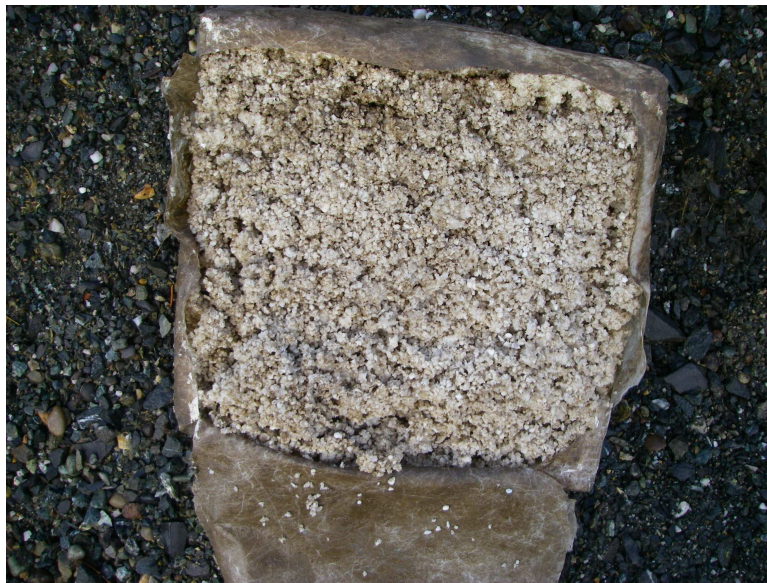
Figure 6. Photograph showing the popcorn like filter matrix inside the Smart Sponge® paks following a period of very high storm water flows. Note the accumulation of fine sediments within the filtration matrix.
