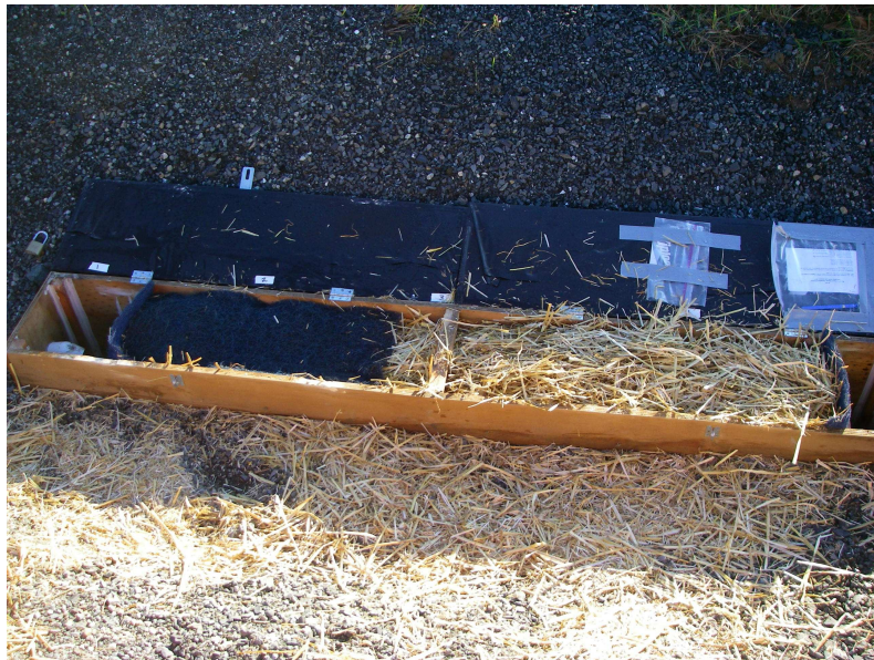
Figure 4. Following clogging of the Smart Sponge® Paks with sediment during a heavy rainfall, a second experiment was set up to test the ability of straw to act as a pre-filter for the Smart Sponge® media.
