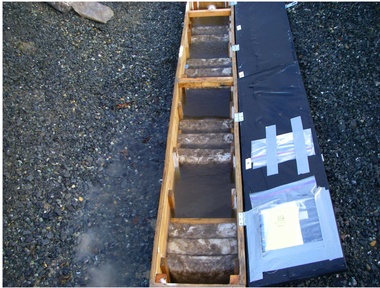
Figure 5. Photograph showing sediments coating the covers of the Smart Sponge® paks following a period of very high storm water flows.
