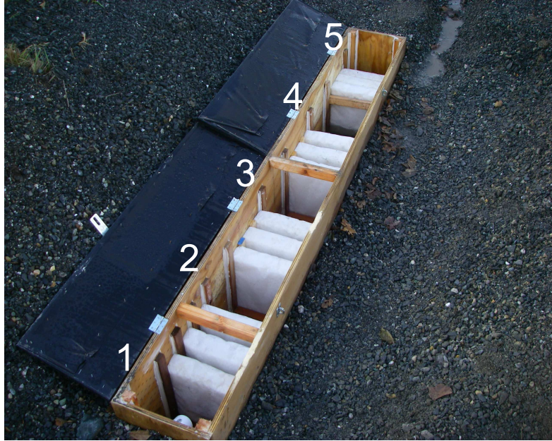
Figure 3. The SWAT experiment trough with the Smart Sponge® paks installed. The design allows the water to flow through up to 12 paks. If the leading paks clog due to sedimentation, then the storm water will flow over the clogged paks to the next sets. The white numbers indicate the locations where coliform and turbidity samples were collected, #1 being the influent and #5 being the effluent.
