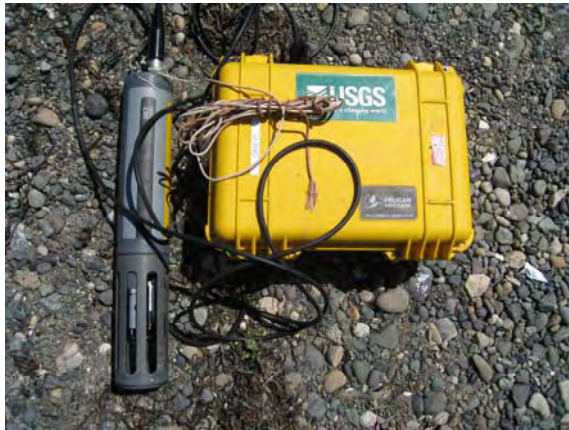
Figure 5. YSI sonde and cables with the Pelican water tight housing.
