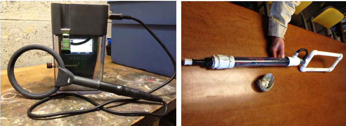
Figure 4. Biomark HPR Plus PIT tag reader contained in a custom Prevco Subsea dive housing, and underwater PIT tag reader developed and constructed by NOAA biologists.
