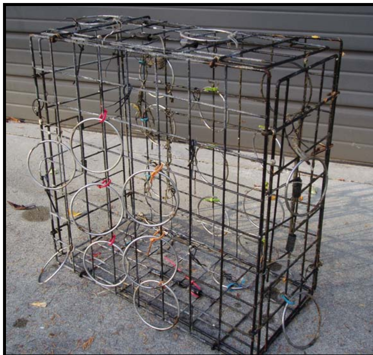
Figure 7. The front panel of pot number 1, with the rings. All the natural cords have disintegrated and the color-coded zip ties show the original placement of the cords.
