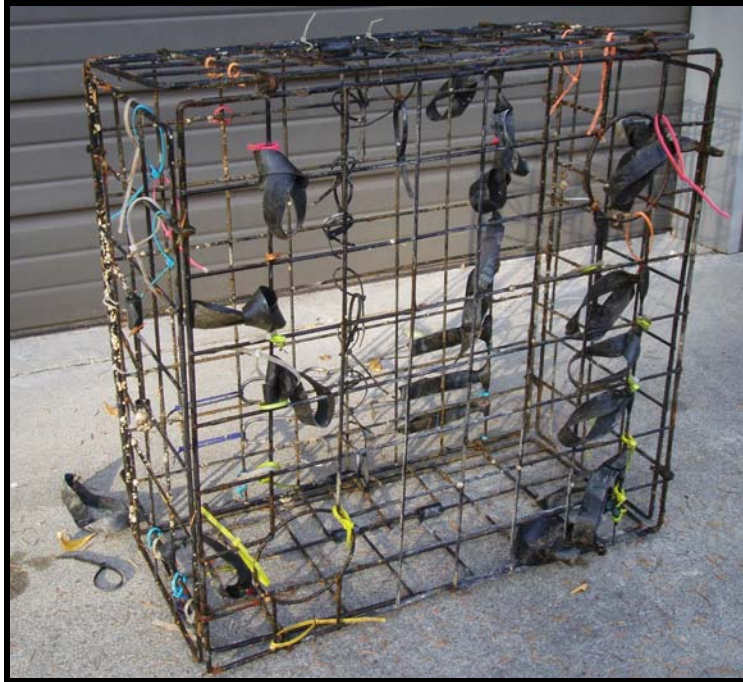
Figure 10. The back side of pot number 2. All the natural cords have disintegrated and the color-coded zip ties show the original placement of the cords.
