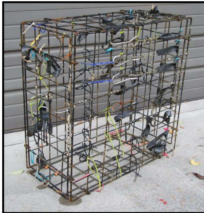
Figure 9. The front side of pot number 2, with the rubber straps. The cotton polyester cords are still present, and are on straps in the upper right quarter of the pot. All the natural cords have disintegrated and the color-coded zip ties show the original placement of the cords.
