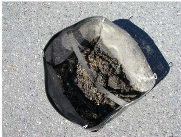
Figure 8. Photographs of the debris collection baskets from each of the Anacortes Smart Sponge ® units sampled on 29 May 2009, one month following installation. Upper left: Anacortes Depot, Upper right: Anacortes Cinema parking lot, Lower left: (9th & Commercial Ave., Lower right: Anacortes Senior Center parking lot.
