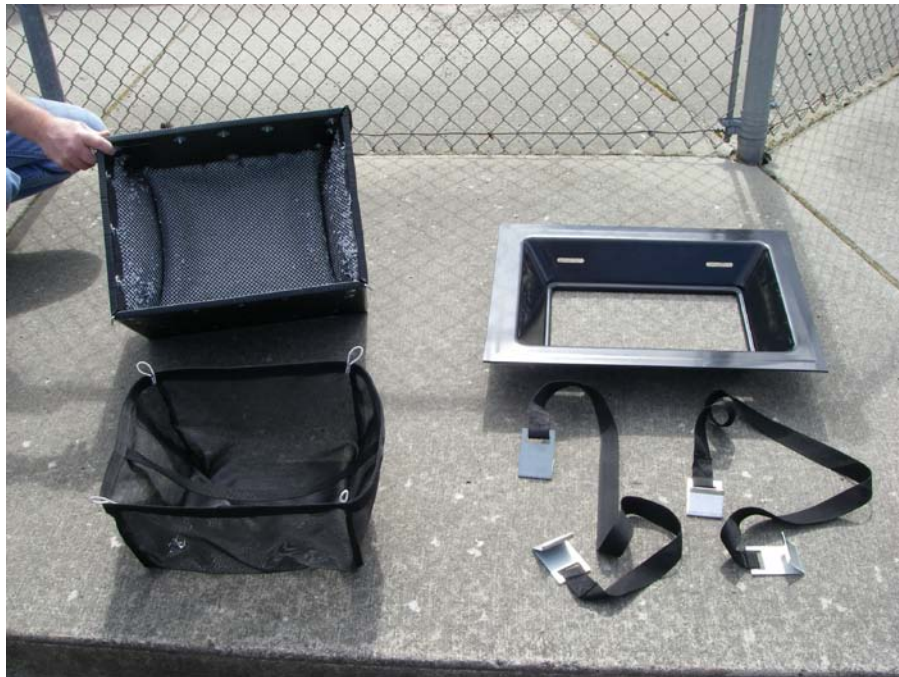
Figure 4. Components of a Smart Sponge ® storm drain filter unit. Upper left: filter box containing the Smart Sponge ® media; lower left: the sediment and debris pre-filter liner (“maintenance saver”); upper right: mounting collar that supports the filter basket and; lower right: mounting straps that connect the basket to the mounting collar.
