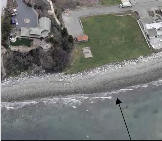
Figure 16. Air photo of Sunset Beach site, note toppled and infringing riprap at west end of site (Pictometry International Corp 2004)
