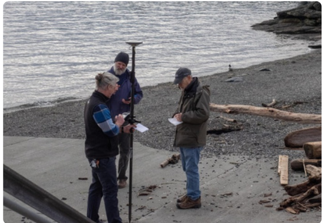
Jeff, Barney Burke, and Dave Wilkinson photographing a small storm surge event in Port Townsend (left); Ian Miller, Jonathan Waggoner and Dave using high resolution GPS to map the Salmon Club boat ramp elevation - photo by Jeff Taylor (right).
